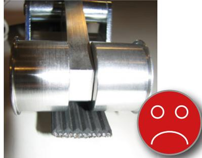
After installation, the correct sensor adjustment should be verified, to ensure that the sensor has been fitted with the right force. The clamping force is correct, if the edge of the adjustment screw's silver cylinder is positioned in the center of the green o-ring. If the edge of the silver cylinder is not positioned inside the O-ring the sensor is incorrectly mounted.
