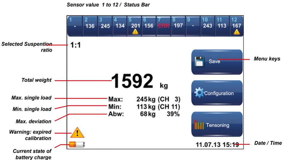
The individual sensor display shows the measured load of each connected rope load sensor.
