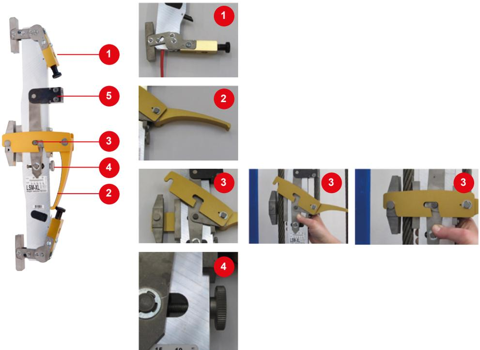
Open both levers 1 as well as lever 2, open strap 3. Adjust the sensor by means of the adjustment screw 4 roughly to the rope diameter and mount the sensor onto the rope. Close strap 3 and after lever 2.
