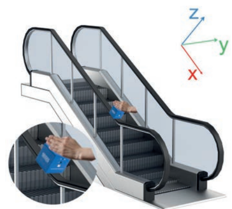
Alignment and positioning of the vibration sensor on the handrails
