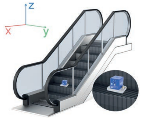
Alignment and positioning of the vibration sensor on the escalator
